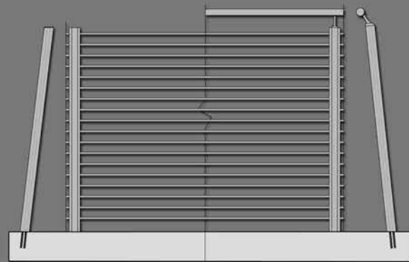
FIXING ON SLAB
